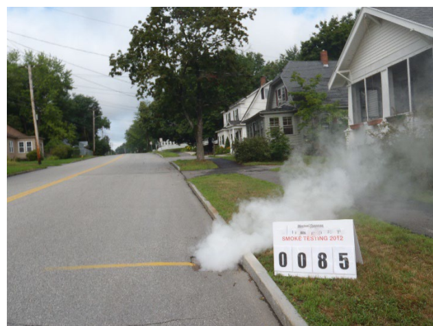
Inflow Source Identified by Smoke Testing
